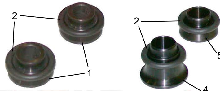
Fit the point C spacers (ref. 1) (top attachment) on the head of the shock absorber.
