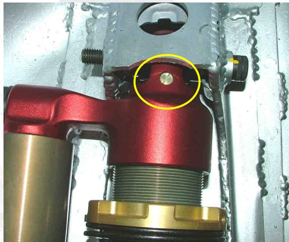
For the right shock absorber, the adjustment screw is turned to the wheelhouse side and is no longer accessible.
