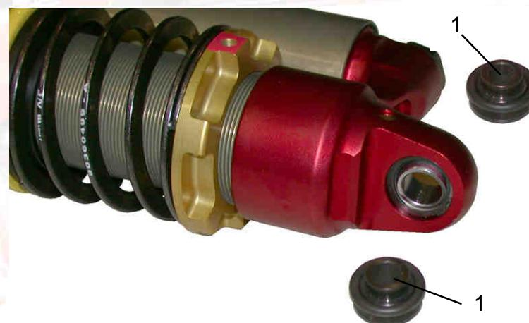
Fit the point D spacers (lower fitting) as indicated below:
